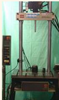
Hydraulic uniaxial testing machine Mod. FPF 20, Italsigma, with a load capacity of 20 kN
