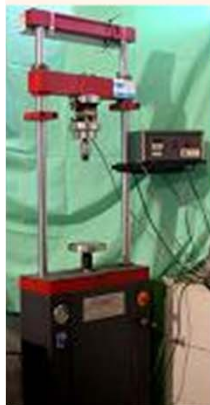
Hydraulic uniaxial testing machine Mod. FPF 20, Italsigma, with a load capacity of 20 kN
