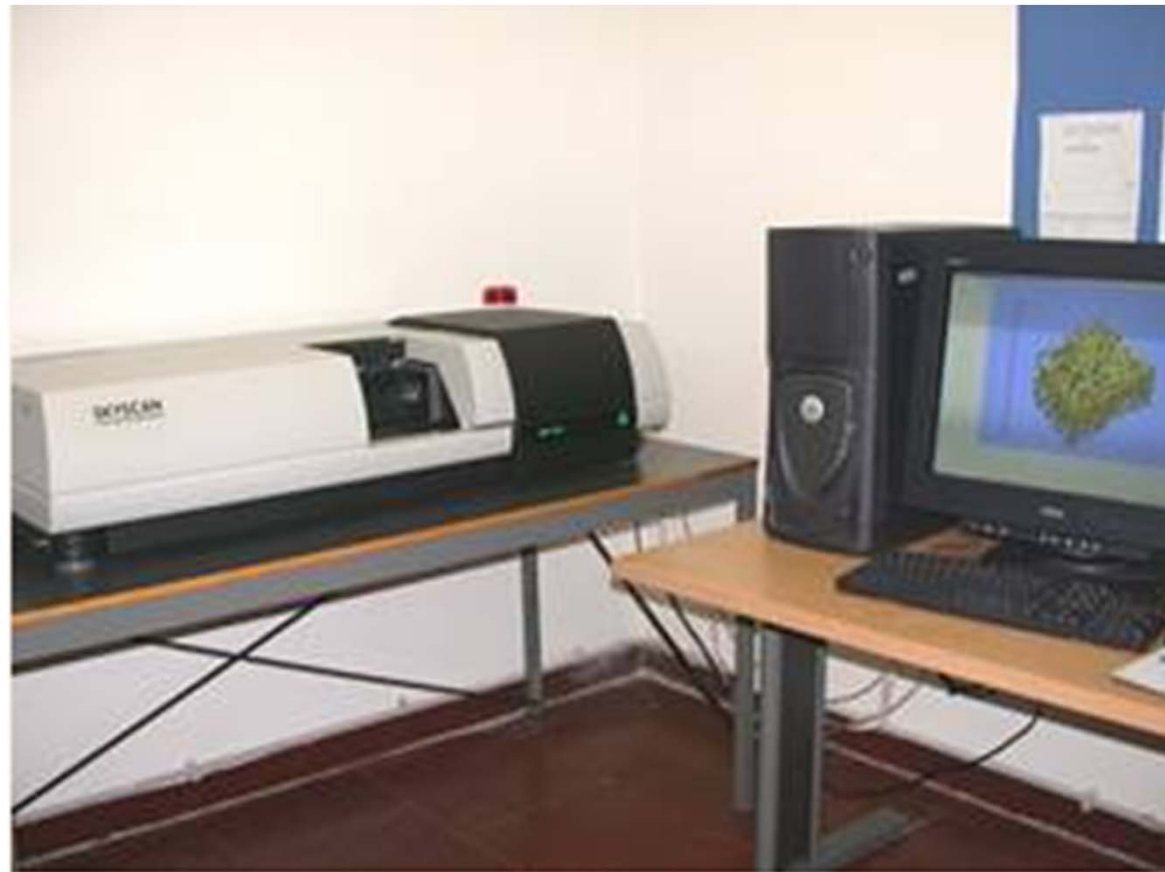
MicroCT system Skyscan 1072 installed at LTM-IOR: Left, microCT system. Right, the external PC
