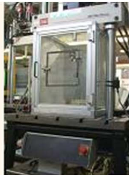
Hydraulic uniaxial testing machine Mod. 8502, Instron, with a load capacity of 100 kN equipped with data acquisition boards (up to 4 channels)
