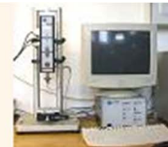
Electric uniaxial testing machine Mod. V1000, Vitrodyne with LOAD CAPACITY OF 100 N
