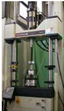
Hydraulic uniaxial testing machine Mod. 8502, Instron, with a load capacity of 100 kN equipped with data acquisition boards (up to 4 channels)
